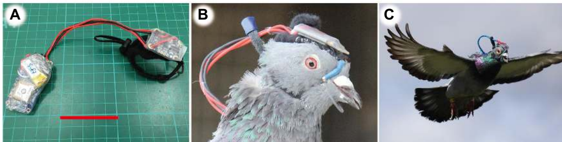
Fig. 1. The 'pSensor' logger. (A) GPS logger, microcomputer, micro-SD card and battery (left; to be carried in a backpack) connected to an inertial measurement unit (IMU) mounted on the custom-made mask (right; to be carried on the head). (B,C) A pigeon wearing the mask and logger.
